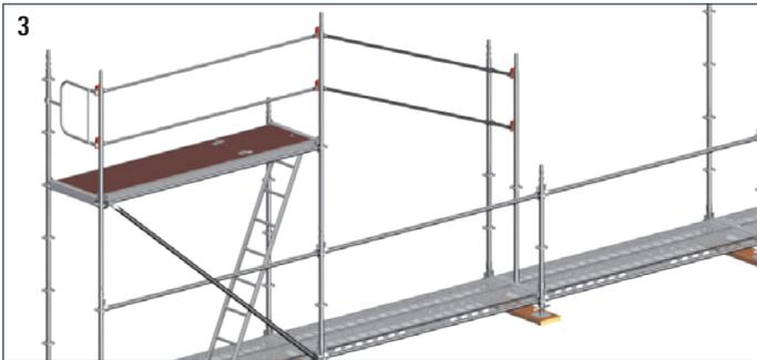
Swing it upwards, fit the AGS standard, install the U-ledger and insert the deck. The entire facade scaffolding can be safely assembled in the same way. Dismantling is in the reverse order.
