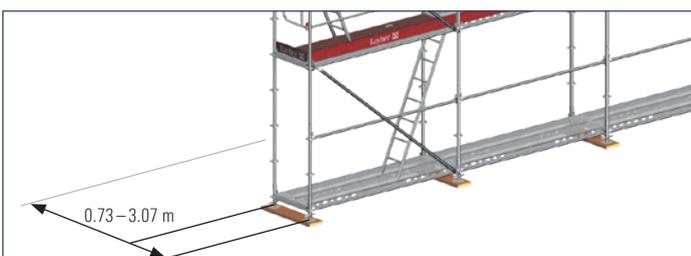
If larger work surfaces are required for reinforcing scaffolding, for example, the scaffolding width can be freely selected up to 3.07 m by using standard U-ledgers or O-ledgers.
