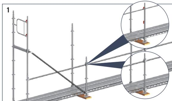
Start at the outside of the scaffolding with 1-metre standards. Fitting the first AGS standard with previously fitted end guardrail. Fitting a U-ledge and an Allround diagonal brace. As an alternative to the base collar and the 1-metre standard, the AGS initial standard LW or the Allround standard LW of 1.16 m with 3 rosettes (see detailed images) can be used.
