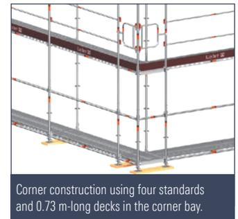
Corner construction using four standards and 0.73 m-long decks in the corner bay.
